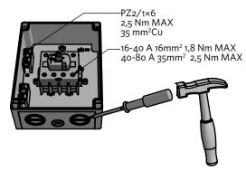
After correct size opening is achieved, insert the conduit/cable connector into the opening from the outside box and secure it using a connector locknut.
