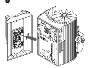
Reinstall the new cover assembly by reconnecting the wiring and reversing the steps to reassemble.
