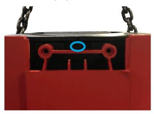
**Step 4:** Install the fan cover with drip cover to the pump. Secure with screw and re-install the cover cap.
