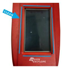
**Step 2:** Remove the lining paper from the back of the LCD cover. Place door over the cover and align center to the touchscreen display. Press along the perimeter of the frame to ensure the double-sided tape is adhering to the cover.
