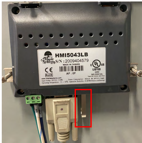
FIGURE 4.1: USB Plugged into HMI
