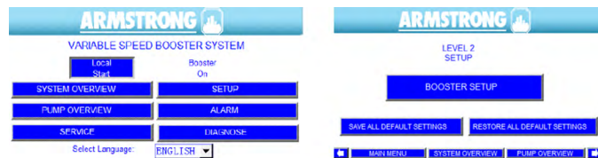
FIGURE 6.1: Booster Home and Set Up Screen
