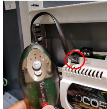
FIGURE 5.2: Smart key - PLC Connection
