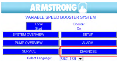
FIGURE 4.7: Booster HMI Home Screen
