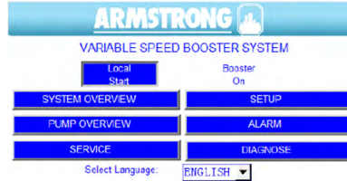
FIGURE 3.1: Booster HMI Main Screen
