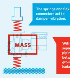
With flex connectors separating the pump from the piping, and vibration isolators between the pump and the ground, the pump floats in an isolated spring system.
