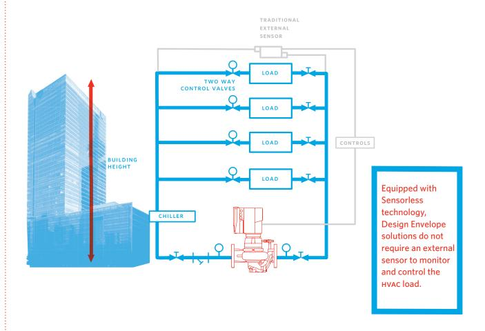
Using Sensorless technology, a Design Envelope pump's performance data (power draw and RPM) and operating curve are pre-programmed into the controller. During operation, the controller monitors the power draw and RPM of the pump and establishes the hydraulic performance and position of the pump's head-flow condition relative to the system requirements.
