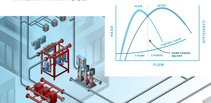
Because HVAC pumping systems mostly operate at partload, a design using two or more smaller pumps is more efficient than one larger pump. In a two-pump system, if one pump fails, the remaining pump can serve the system requirements with up to 70% flow redundancy. The capacity split can be adjusted based on the building type and duty requirement.
