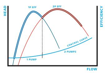
\*PSPC CAN CONTROL AND STAGE UP TO 4 PUMPS The Armstrong IPS 4000w is available to control more than 4 pumps.
