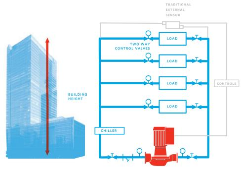
Equipped with Sensorless technology, Design Envelope solutions do not require an external sensor to monitor and control the HVAC load.
