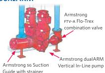
dualARM Vertical In-Line incorporates two pumps in a casing with single inlet and outlet connections. Enables standby or parallel operation with only one set of piping. Casing design and port valves allow one pump to be removed for service with the second pump still operating. When installed with a Suction Guide and Flo-Trex valve the dualARM represents the greatest Life Cycle Value in today's commercial HVAC market.
