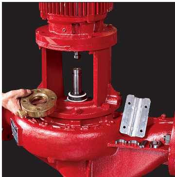
3) Disconnect seal flush line and remove gland plate bolts. The gland plate and seal seat may then be taken out between the space in the shafts. With inside seal the complete seal is removed following the gland plate.
