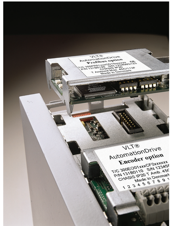
Many option cards simply plug into slots under the drive keypad
