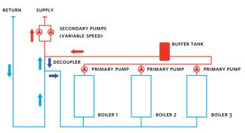
The figure shows a typical constant primary variable secondary system consisting of three boilers running in parallel each having its own circulating pump. The Decoupler, decouples or 'hydraulically separates' the primary (boiler) and secondary (system) loops and prevents flow in one circuit from interfering with the other. Hence as zone valves open, close, or modulate, and as system pumps vary speed, the boiler loop is not impacted.
