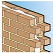
Typical cavity wall construction
