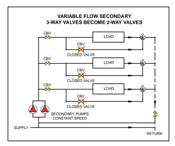
ger be bypassed; thus the loop differential head would increase as the control valve throttles the flow. As this throttling reduces the system flow, pumping power needs are reduced.
