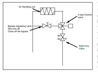
To convert existing 3-way valve systems to 2-way valve configuration is relatively easy. Simply close the regulating valves in the bypass lines. With the bypass closed, when the 3-way valve modulates attempts to divert the flow around the load and through the bypass, it will restrict the flow rate instead. An Armstrong IVS Sensorless pump will sense this deviation from its control curve and reduce speed until the pre-set control curve, the system resistance curve and the pump perfor-
